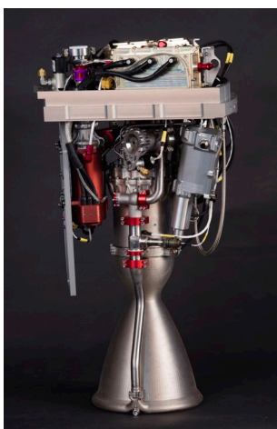
Figure 2 First Stage Rutherford Engine
