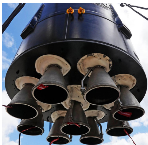
Figure 3 Rutherford Stage 1 Configuration
